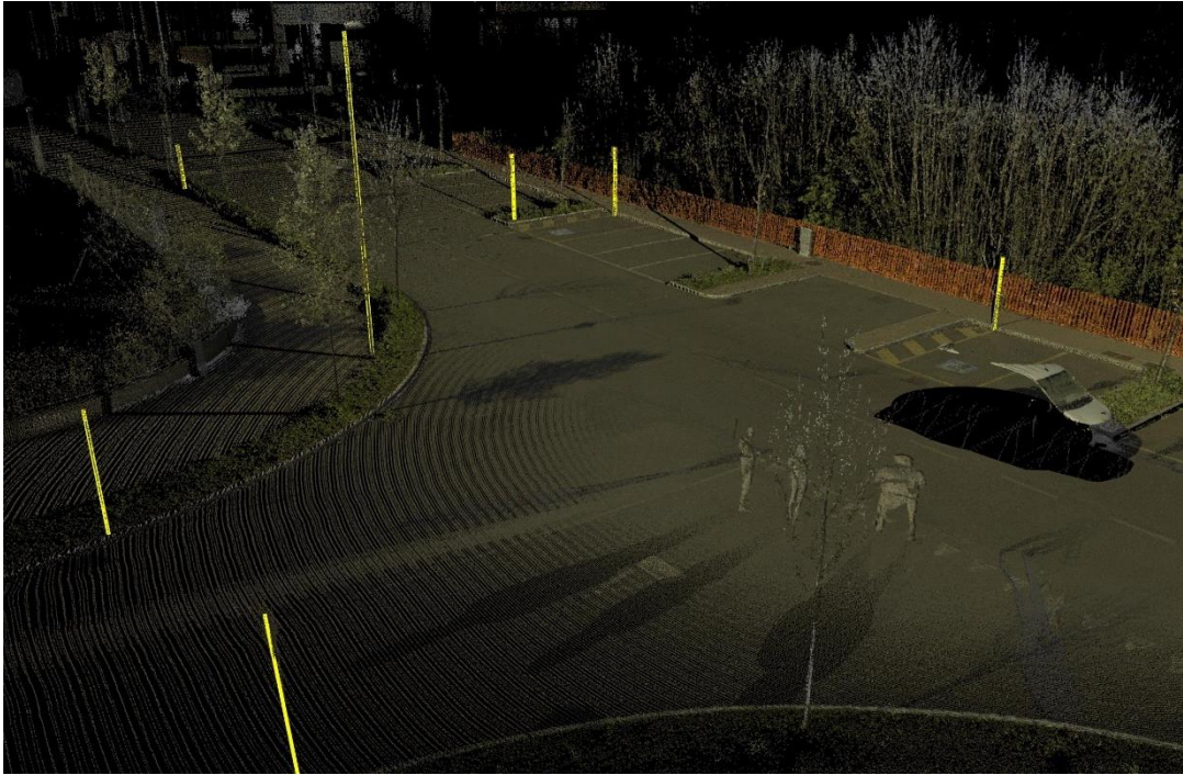
Axis of poles extracted in 1-click from Line Region Grow with OK, Next capacity
