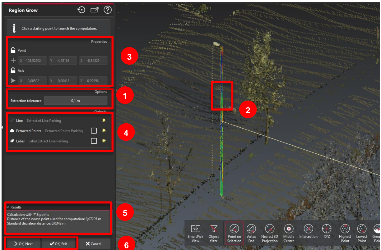
Pole Best Line extraction from a single click in the 3D Scene
