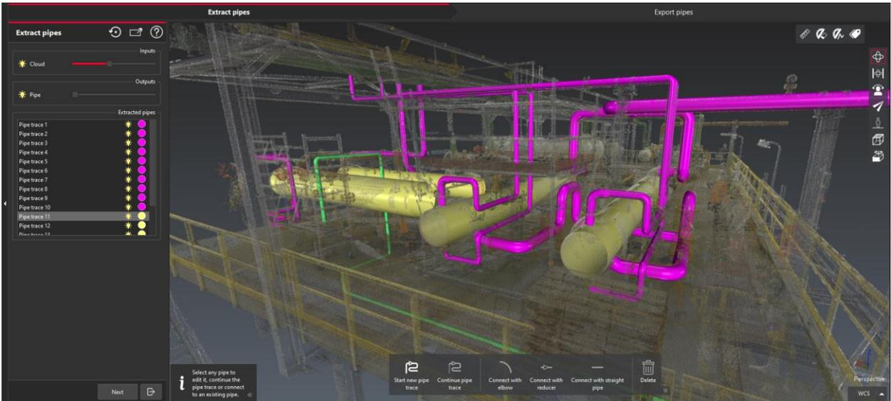
Example of a chemistry plant site extracted from 3DR Scan to Pipe
