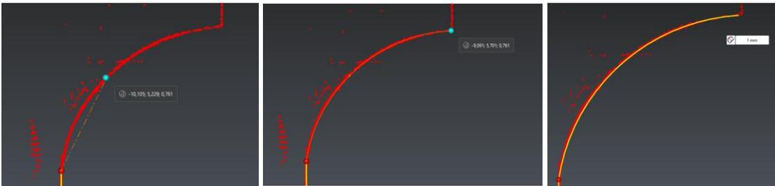
The “Tangent” arc method requires 1 additional click from the extremity of the polyline segment and the arc curve direction is tangent to the latest segment:
