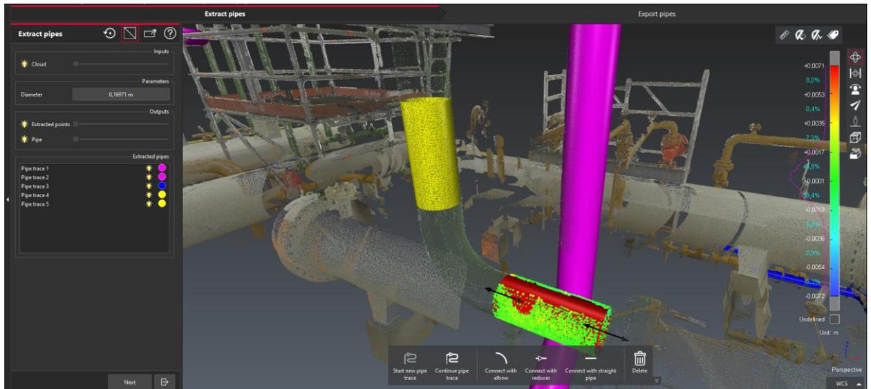
*The 2 segments will be connected with an elbow.*
