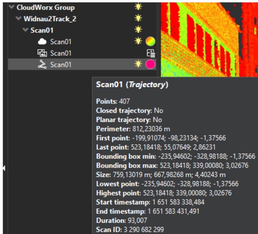
Many existing features are compliant with scanner trajectory with a similar behavior to polyline:
