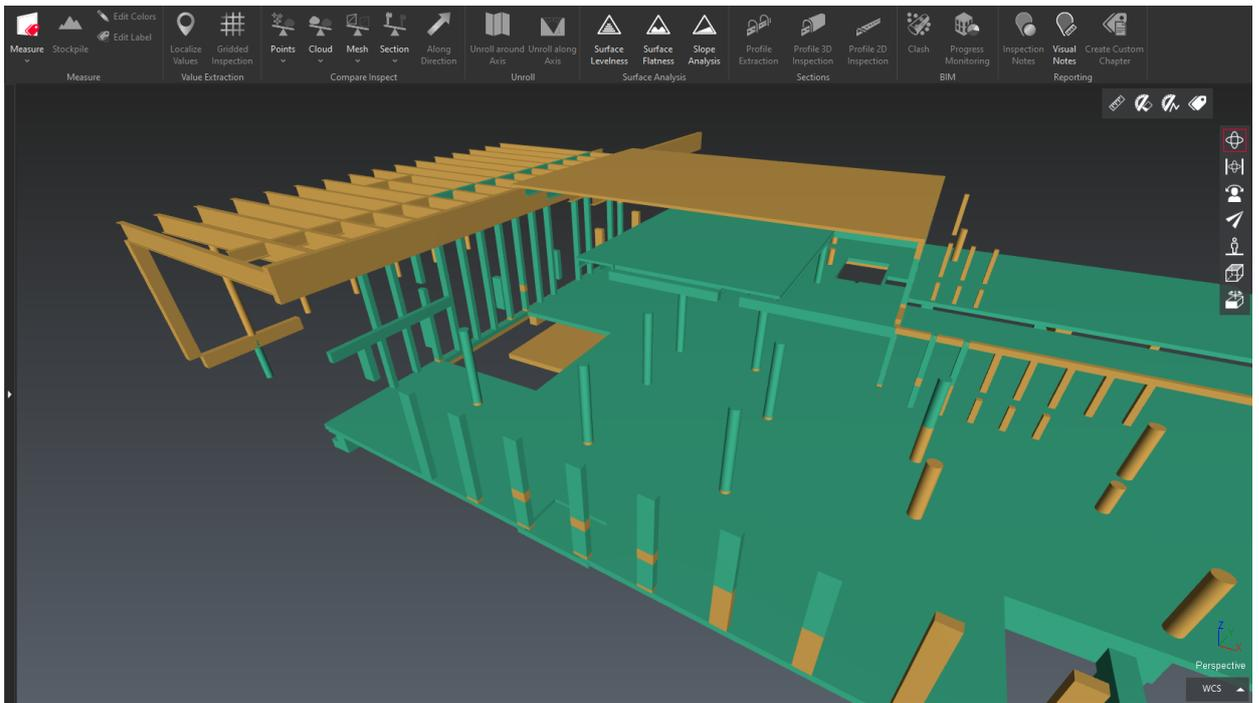
In this progress monitoring analysis, only the “Installed” and “Incomplete” components are displayed to simplify the visualization experience. It is extremely easy to filter the components with the updated treeview management of the feature.
