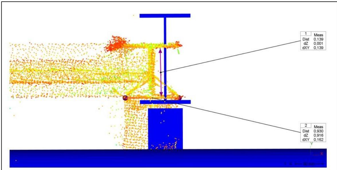
*Example of an issue in the structural design explained with 2D measurements to illustrate the gap between the design model and the reality for the dimensions of the steel column*
