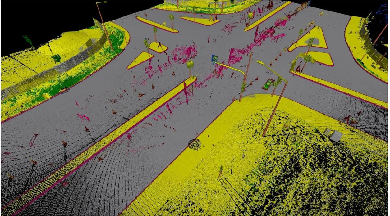
*Point cloud of a road intersection captured with RTC360, classified with the new ROAD model*
