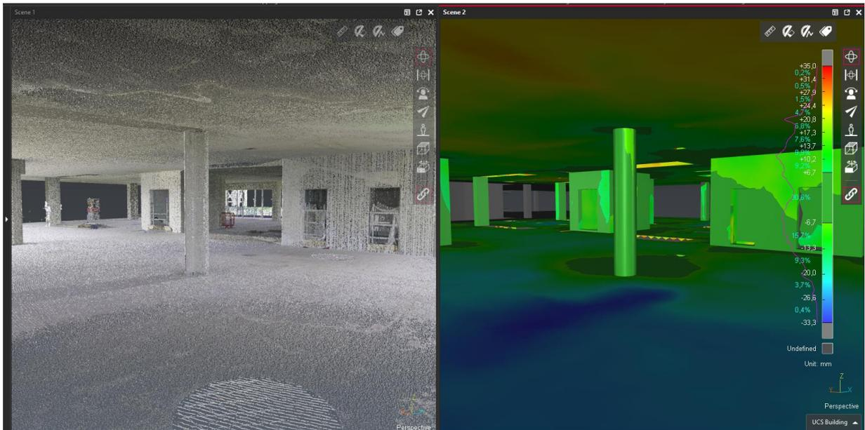
*The 3D environment is displayed on two synchronized 3D views after a click on Compare side by side. In this example, the colormap from a BIM Inspection analysis and the original point cloud are displayed.*
