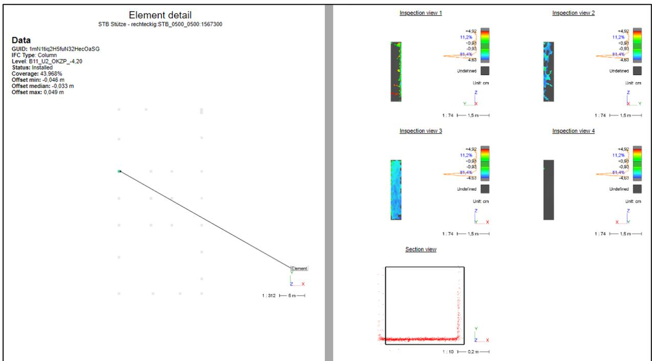
Report extract of a column that is installed but slightly shifted from the design model.
