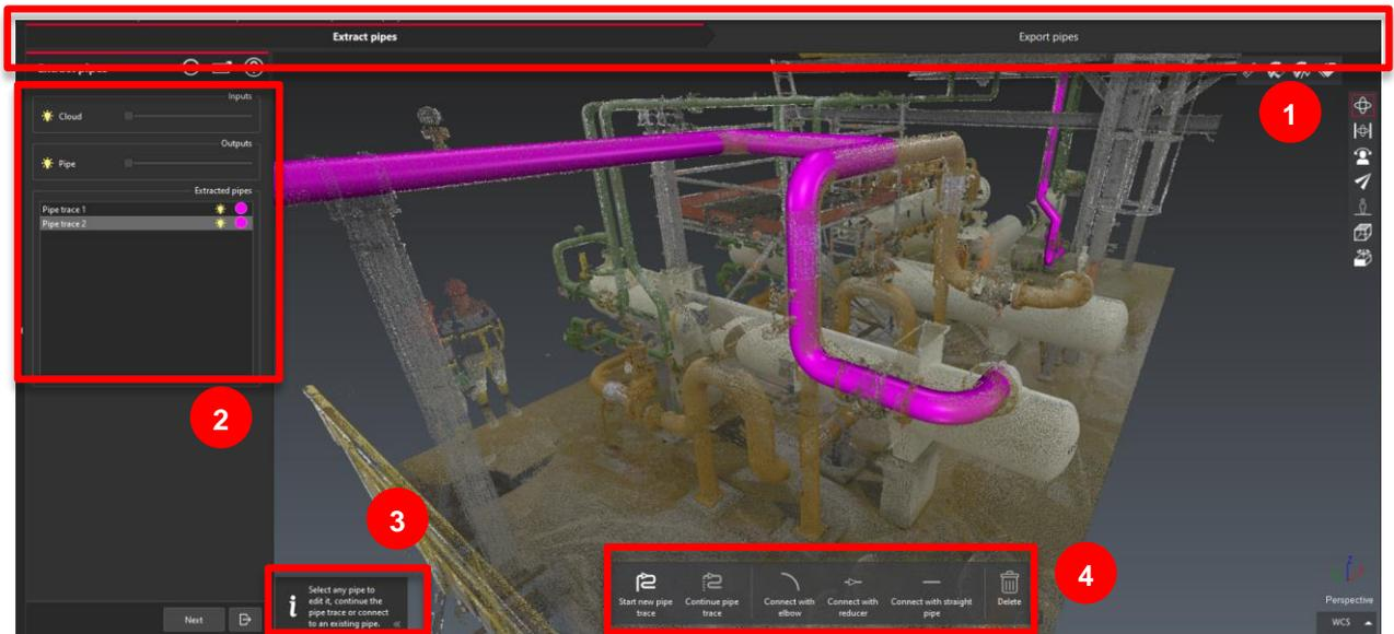
1. **Workflow ribbon:** showing the 2 steps of the workflow. It is possible to switch from one step to another one from the ribbon.
