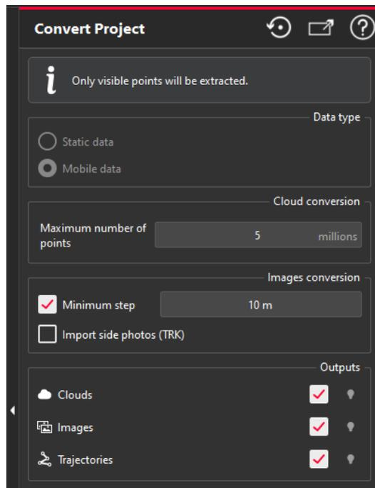
For LGS/LGSx point cloud with a trajectory (Mobile BLK or TRK scanners), there is a specific option to extract camera images at a minimum step. To be defined by the user according to the targeted application (for example, every 2 meters for Indoor – every 15 meters for an MMS scan).
