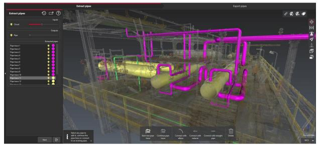
Example of a chemistry plant site extracted from 3DR Scan to Pipe
