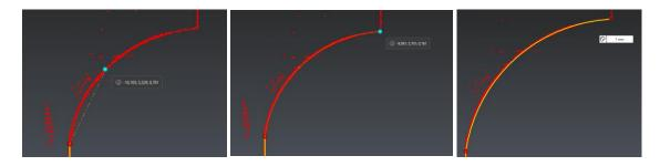
The "Tangent" arc method requires 1 additional click from the extremity of the polyline segment and the arc curve direction is tangent to the latest segment:
