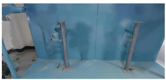
Cyclone 3DR 2024.0: WITH filtering capacities. The textures of the pipes are not projected on the background wall anymore.
