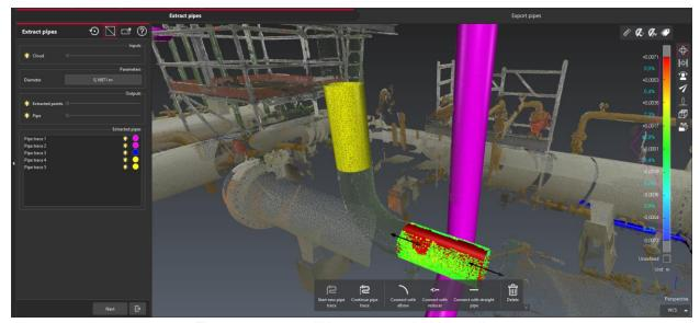
The 2 segments will be connected with an elbow.
