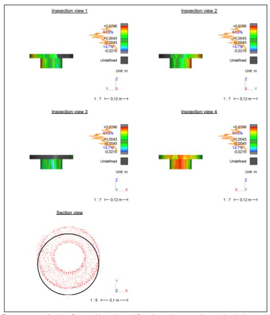
Report extract of a pipe-flange with a ~3 cm shift to the top in comparison to the design model
