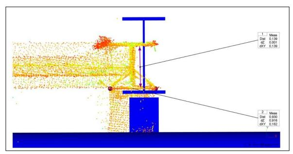
Example of an issue in the structural design explained with 2D measurements to illustrate the gap between the design model and the reality for the dimensions of the steal column
