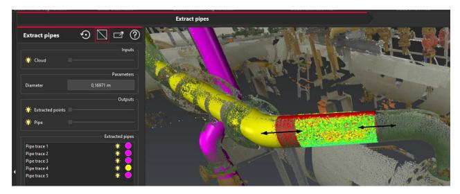
• **Reducers:** like straight pipes, the 2 diameter values can be edited, and the arrows give the opportunity to adjust the length of the reducer. The offset can also be edited but only if the reducer has one free extremity. The offset value is 0 if the reducer is a symmetric one.
