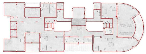
Floorplan from an office building captured with BLK2GO and extracted with the upgraded Scan to Plan in Cyclone 3DR 2024.0
