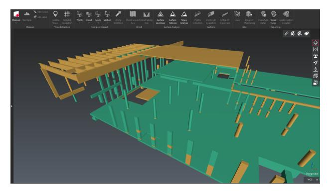
In this progress monitoring analysis, only the "Installed" and "Incomplete" components are displayed to simplify the visualization experience. It is extremely easy to filter the components with the updated treeview management of the feature.
