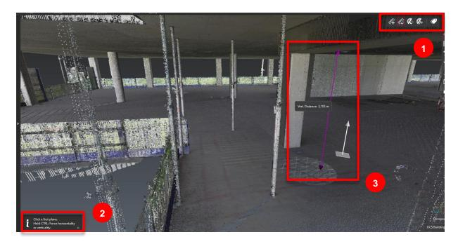
The height under the beam can be measured in Cyclone 3DR for this scanned construction area.
