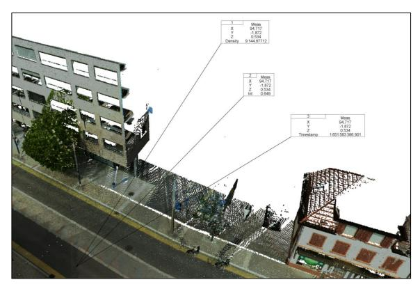
Different labels extracted from the TRK scan of the road (Density / Intensity / Timestamp)
