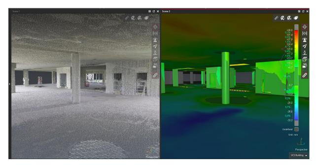
The 3D environment is displayed on two synchronized 3D views after a click on Compare side by side. In this example, the colormap from a BIM Inspection analysis and the original point cloud are displayed.
