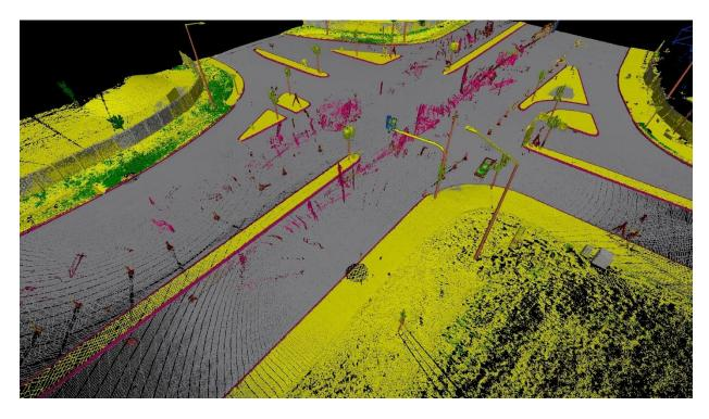
Point cloud of a road intersection captured with RTC360, classified with the new ROAD model
